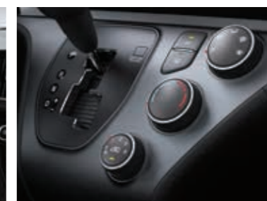
Manual air conditioning system
