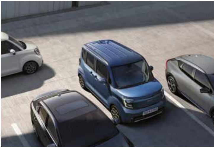
Rear Cross-traffic Collision-avoidance Assist Alerts the driver if a car is approaching the back from the left or right while pulling out in reverse. Automatically helps to brake the car if the risk of colliding increases even after sounding an alarm.
