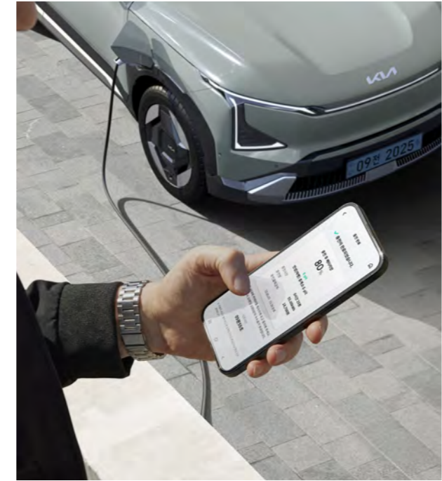
Automatic Charging Payment System (PnC) Without authentication at E-pit charging stations, charging starts by plugging into the charging inlet port, with automatic payment when charging is complete. *PnC : Plug & Charge
