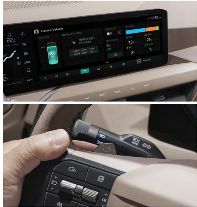
Battery State Information (Charge-Discharge Pattern Analysis) Battery capacity analysis allows available range, battery charge level and charging type for more efficient battery management. i-PEDAL 3.0 At all stages of regenerative braking, the accelerator pedal can be used to adjust the car's speed or stop it. A memory function is available for reverse parking and restarting. ※ The reverse parking function can be switched on or off in the system settings menu.
