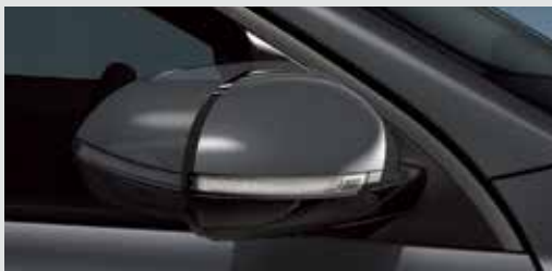
Auto folding outside mirrors (SX only) Outside mirrors can auto-fold to fit into tight parking spaces.
