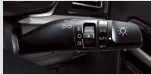
Auto light control Set the stalk control to Auto and the headlights and tail lights will come on automatically at dusk or in dark places.
