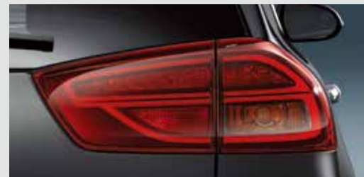
LED rear combination lamps The rear combination lamps use energy-efficient LEDs for immediate illumination and consistent brightness.
