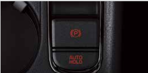
Electronic Parking Brake (EPB) (SX only) When stopped on a steep incline, use the EPB Auto Hold button, mounted in the center console, to prevent the vehicle from rolling back.
