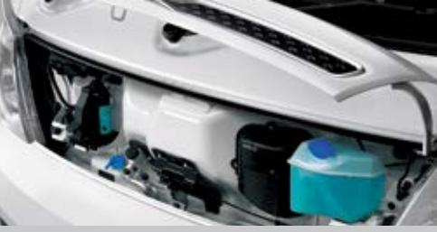
**Front open panel:** Allows you to easily check fluid levels and refill when necessary.
