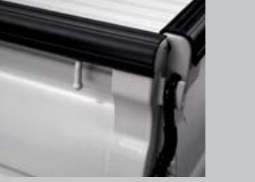
**Round-edged brim cover:** Allows for easier loading and unloading, as well as greater durability.
