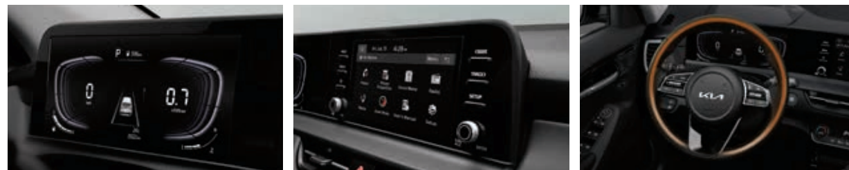
Supervision cluster (4.2-inch color TFT LCD)
