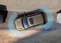
Parking Distance Warning (PDW) With ultrasonic sensors mounted on the front and rear bumpers, PDW warns of any obstacles when you maneuver into tight spaces.
