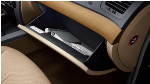
Glove box: The large-sized glove box compartment provides enhanced convenience and sophistication. It features a locking mechanism for safekeeping of items, a lamp to help illuminate items in the dark and a damper for smooth and controlled opening.
