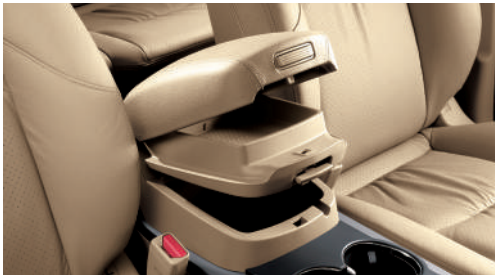
Centre console: The centre console is far more than a comfortable armrest. Beneath is a spacious storage box, mounting for the rear ventilation ducts, and a cup holder.
