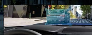
**Forward Collision-Avoidance Assist (FCA)** FCA uses a front-view camera and front radar to detect vehicles, pedestrians or cyclists ahead. By warning the driver and automatically applying the brakes, FCA helps to avoid or reduce the severity of an accident.
