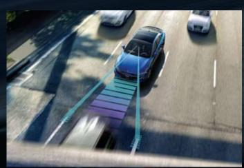
**Smart Cruise Control (SCC)** SCC maintains the driver's selected speed and, using the front-view camera and front radar, helps to maintain a safe following distance. SCC will reduce speed and even stop the car when needed. Then when the car ahead moves, SCC automatically accelerates for you. SCC is now activated with the simple touch of a button.
