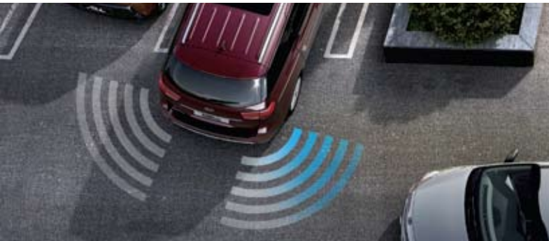
Rear Cross-Traffic Alert (RCTA) When backing out of a parking spot or driveway, the system warns the driver if it detects any cross traffic in the lane the vehicle is entering.
