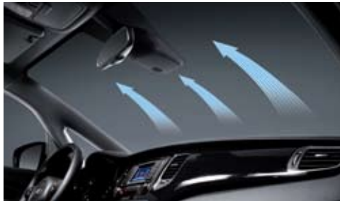
Auto defogging system A sensor automatically initiates a defogging process when condensation is detected on the windows to ensuring optimal visibility in humid climates.
