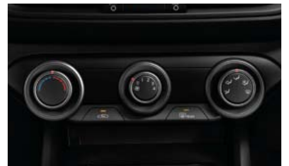
Manual temperature control
