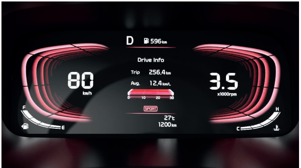
Full Segment LCD Cluster with Advanced 10.6 cm (4.2") Color TFT MID
