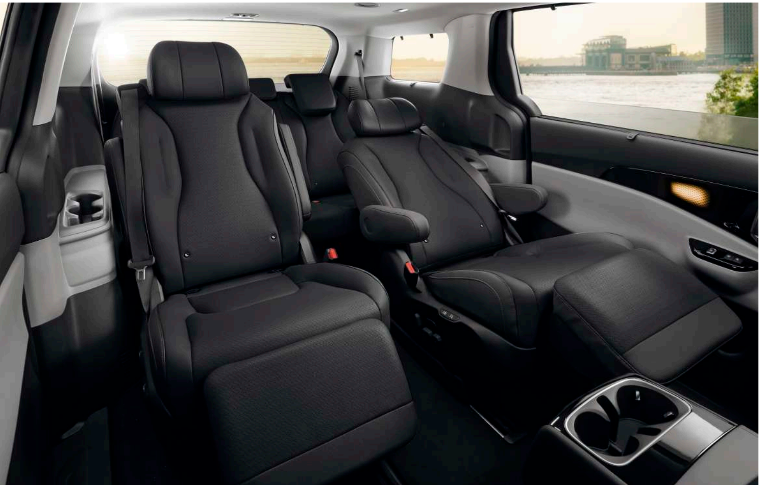
Relaxion Seats with Center Walk Through, Long/Lateral Sliding, and 8-Way Power with Heating, Ventilation and Memory Functions
