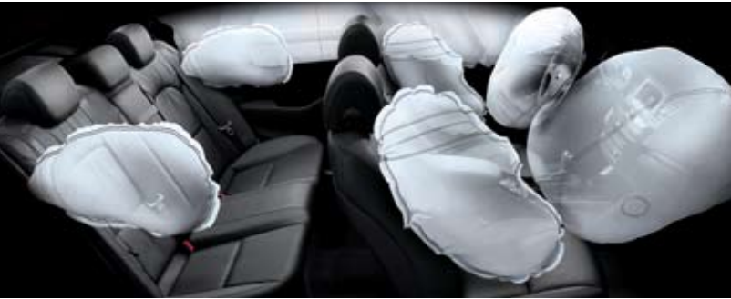
8-airbag System Dual front, twin front seat side and full-length curtain airbags, plus twin rear seat side airbags, provide an exceptional level of protection for all occupants while an intelligent airbag mechanism ensures deployment at an appropriate pressure to prevent excess injury.
