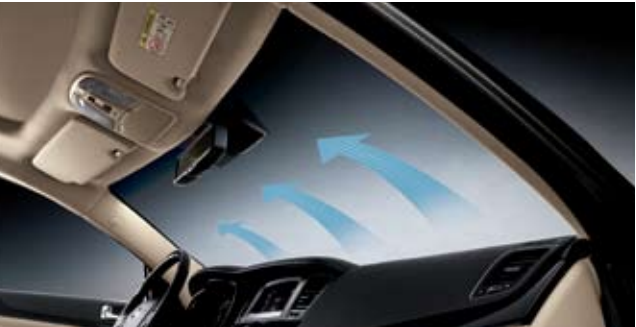
Auto Defog System Sensors detect any condensation that forms on the inside of the front windshield and automatically turn on the defogger for maximum visibility and safety.
