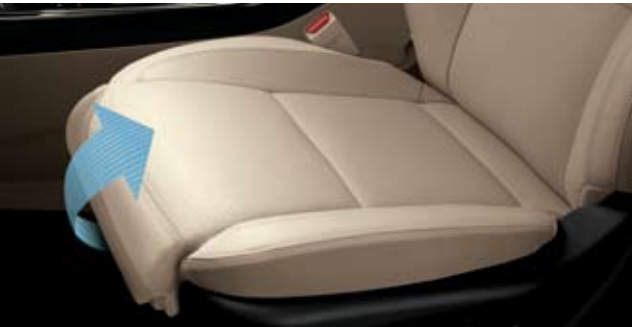
Driver Seat Knee Extension Designed for long-legged drivers, the bottom cushion of the driver's seat can be extended forward at the push of a button for optimal driving comfort.
