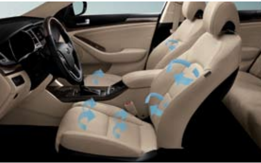
Ventilated Seats Cool air is channeled and discharged through both the driver and front passenger seats via inner-mounted air ducts to prevent perspiration in hot weather conditions.
