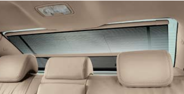
Power Rear Sunshade A convenient one-touch mechanism lowers or raises the automatic rear glass curtain for better privacy while helping keep the cabin cool on hot summer days.
