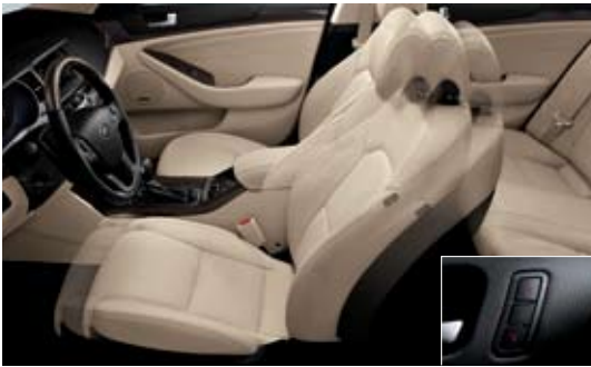
IMS (Integrated Memory System) A smart memory function remembers your preferred driving position and automatically adjusts the 8-way power driver seat, steering wheel and outside mirrors.
