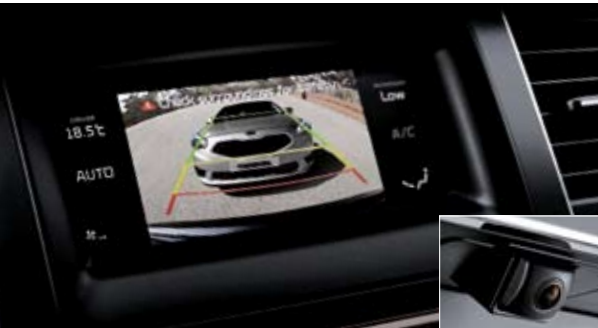
Rear View Camera Backing up and parking in tight spaces has never been easier. The center fascia monitor gives you a clear view of any obstructions behind your vehicle.
