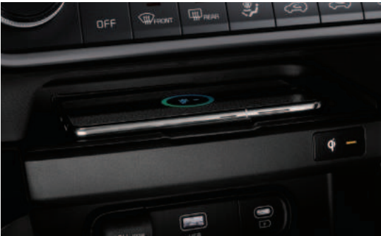
Wireless charging tray The charging pad in the dash, in front of the center console, lets you quickly charge compatible mobile phones, wirelessly.
