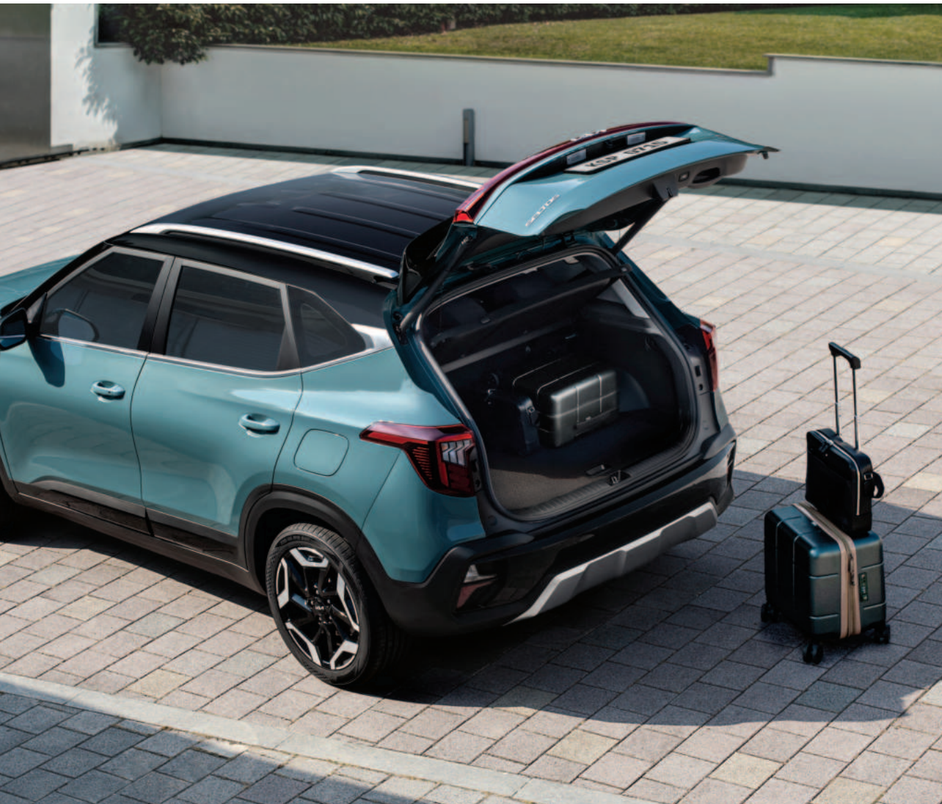
Power tailgate The power tailgate can open and close automatically. The electro-mechanical system works with a wireless remote key fob or by hand, using the outside handle or a touch-button switch just inside the tailgate.
