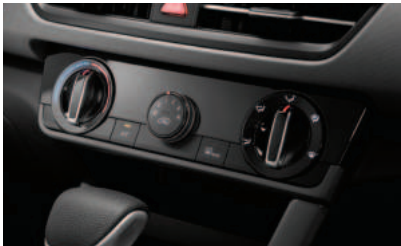
Manual temperature control
