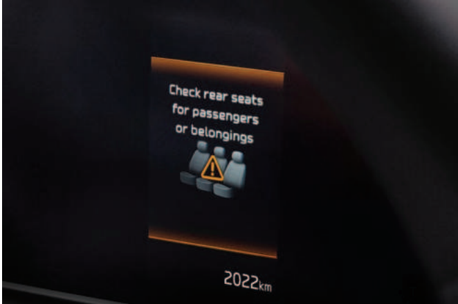
Rear Occupant Alert (ROA) To make sure no one is left alone, ROA warns you of any rear occupants when you stop and prepare to exit.
