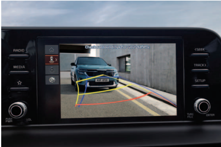
Rear View Monitor (RVM) The Rear View Monitor displays video of the situation behind the vehicle for safe parking.
