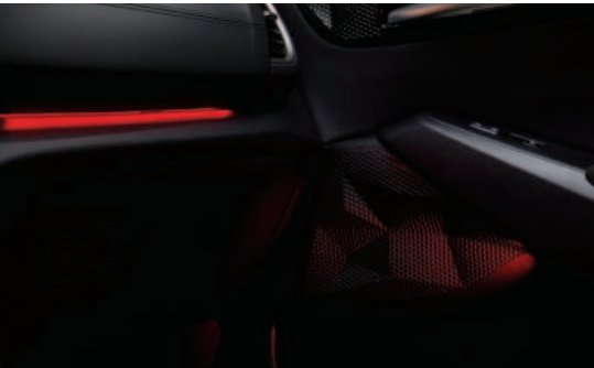
Ambient light Mood lighting on the door speakers and crash pad garnish changes in brightness in synchrony with the audio system sound.
