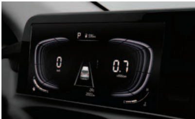
Supervision cluster (4.2-inch color TFT LCD)
