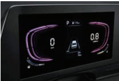
Supervision cluster (4.2-inch color TFT LCD)
