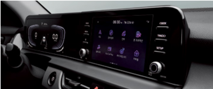
Supervision cluster (4.2" color TFT LCD) & 8" display audio
