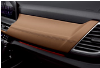
Crashpad in-mold stitching
