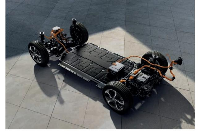
**Electric Global Modular Platform (E-GMP).** The Kia EV6 is the first vehicle based on the Kia E-GMP platform. The new longwheelbase platform is a clean slate. It introduces a flat floor, facilitating new comfort and utility choices. Its modularisation gave our engineers more options to meet tough performance, maintenance and safety objectives. In terms of performance, their aim was to achieve greater power, driving range and control, as well as shorter charging times.
