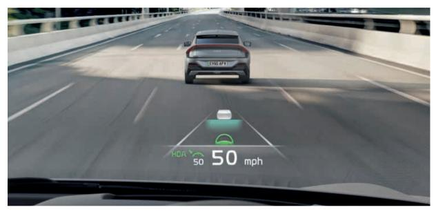
**Augmented Reality head-up display.** The Kia EV6's head-up display projects driving information on the windscreen. It superimposes turn instructions from the navigation system over the roads ahead, lets you know if you're drifting out of your lane and indicates which vehicle is detected ahead of you (grade dependent).
