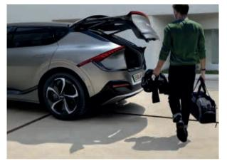
**Smart power tailgate.** The power tailgate can be set to open automatically to a desired height.
