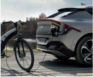
**Vehicle-to-load (V2L).** Get 220 V of alternating current to power your devices, inside or outside the Kia EV6. Fully charged, its vehicle-to-load feature offers 3.6 kW of power, enough to run a large TV screen or a medium-sized air conditioner for 24 hours. Inside the Kia EV6, just select EV Ready or Utility mode and use the outlet at the base of the rear seat. Outside, simply attach the vehicle-to-load connector to the charging outlet (grade dependent).
