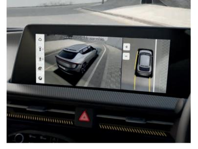
**Surround View Monitor.** Gone are the days when you need to exit the vehicle or ask others for help with tricky manoeuvres. Images from four cameras are synthesised to give you a 360° 3D view around the vehicle, so you can steer and park with confidence (grade dependent).
