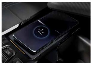
**Wireless phone charger.** The charging pad in the front centre console lets you charge compatible mobile phones wirelessly. It operates with up to 15 W of power, so charging is reassuringly fast (grade dependent).
