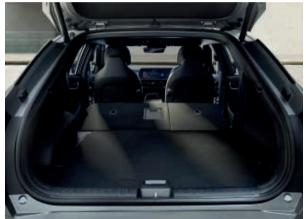
**Remote second-row seatback folding.** Pull the remote release lever on the wall of the cargo space to fold the rear seatback down, creating 1,300  $\ell$  of storage capacity. With the lever's convenient location, it's like having an extra pair of hands when you need to load long or bulky items.
