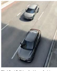
Blind-Spot Collision-Avoidance Assist. When you signal a lane change, you are warned if a risk of collision is detected with a vehicle beside you or approaching from the rear. The system even interacts with your steering if the risk increases. Blind-Spot Collision-Avoidance Assist also watches out for you when pulling out of parallel parking spaces, warning you about oncoming traffic behind you (grade dependent).
