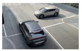
Forward Collision-Avoidance Assist with junction turning and crossing. It uses a front-view camera and radar to detect any vehicles, pedestrians or cyclists ahead. By warning and braking automatically, it can help you avoid, or reduce the severity of an accident. The system also engages when you are crossing or turning at an intersection (grade dependent).
