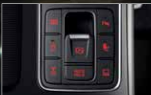
Drive mode select system By pressing a button you can choose between Normal, Eco or Sport drive mode to adjust the transmission shift points to your preferred driving style and the driving environment: Normal for everyday driving, Eco for more fuel efficient gear changes and Sport for a more dynamic drive. Standard on automatic transmission models.
