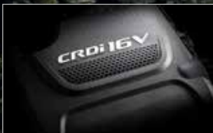
2.2 CRDi diesel engine Max. power 200 PS @ 3,800 rpm
