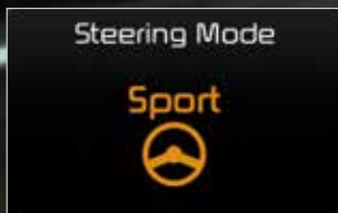
Flex steer system Choose from three modes to adjust the steering response and effort to different road conditions: Normal for regular conditions, Comfort with lighter steering for urban driving and easy parking and Sport for a more engaging drive on the motorway. Standard on manual transmission models.
