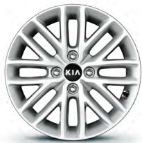
Alloy wheel kit 15". Eight double-spoke alloy wheel, 6.0Jx15, suitable for 185/65 R15 tyres. Kit includes a cap and four nuts. H8F40AK000 (MY17)
