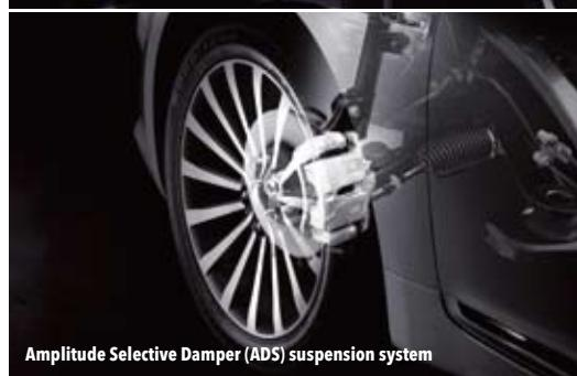
Amplitude Selective Damper (ADS) suspension system
