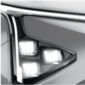
Star Map LED DRLs with Integrated Turn Signal and Ice Cube MFR LED Headlamps
