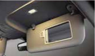
Sunvisor illumination lamps LEDs over the vanity mirror on the driver-side sunvisor light up to help you see yourself better in the mirror.
