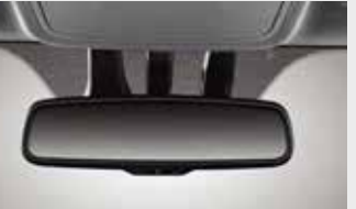
ECM rear-view mirror The Electro-Chromic Mirror automatically controls the glare from the headlamps of the car behind you in nighttime.
