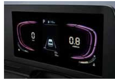
Supervision cluster (4.2-inch color TFT LCD)
