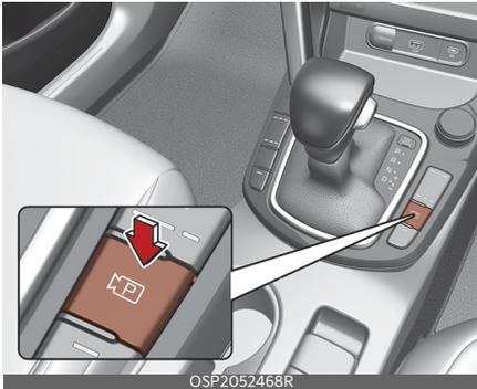
Press the Parking/View button (1) to turn on Rear View Monitor.
