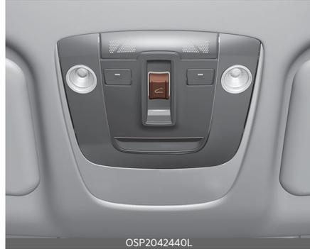
The sunroof can only be operated when the ignition switch or the ENGINE START/STOP button is in the ON or START position. The sunroof can be operated for approximately 3 minutes after the ignition switch or the ENGINE START/STOP button is in the ACC or LOCK/OFF position. However, if the front door is open, the sunroof cannot be operated even within the 3 minutes period.
