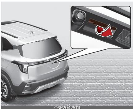
When the tailgate is closed, press the power tailgate open/close switch to open the tailgate.
