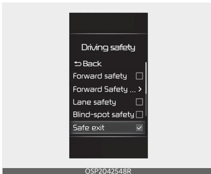
With the ignition switch or ENGINE START/STOP button in the ON position, and select 'User settings → Driver assistance → Driving safety → Safe exit' on the instrument cluster or 'Settings → Vehicle → Driver assistance → Driving safety → Safe exit' on the infotainment system.
