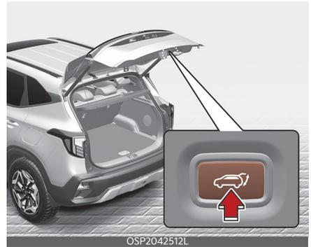
Press the power tailgate open/close button. The tailgate opens or closes with a warning sound.
