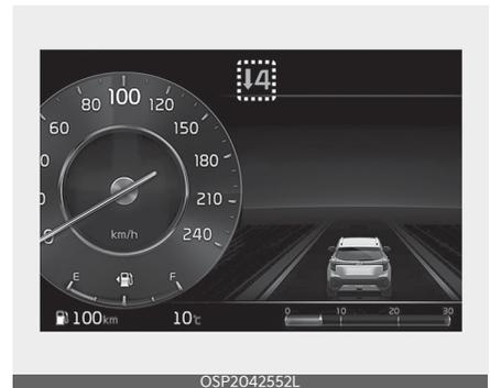
This indicator informs which gear is desired whilst driving to save fuel.
