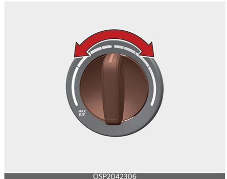
To change the air temperature in the passenger compartment, turn the knob
