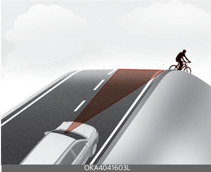
Forward Collision-Avoidance Assist may not detect other vehicle, pedestrian or cyclist in front of you whilst driving uphill or downhill adversely affecting the performance of the sensors.
