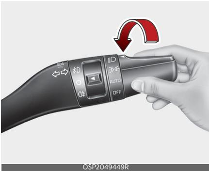
When the light switch is in the head light position, head light (low beam), tail, license light will turn ON.
