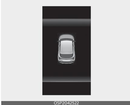
The warning chime will operate when the vehicle is being driven at or above 7 km/h (4 mph) with the bonnet open.
