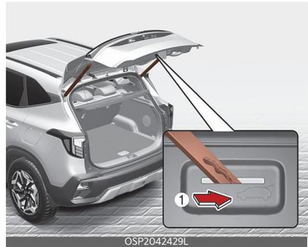
To unlock and open the tailgate manually from inside the luggage compartment, perform the following procedure:
