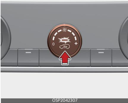
To change the air intake control position. The air intake control is used to select the outside (fresh) air position or recirculated air position.
