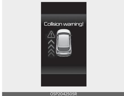
The warning light on the side view mirror will blink and the warning message will appear on the cluster, and an audible warning will sound.
