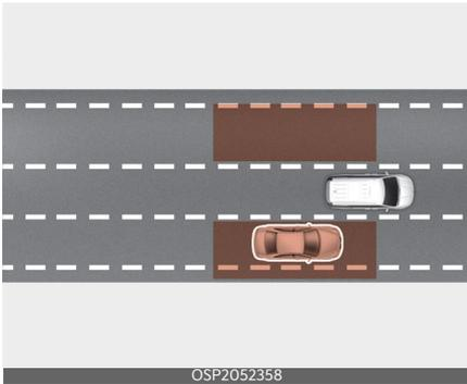
Blind-Spot Collision-Avoidance Assist helps detect and informs the driver that a vehicle is in the blind spot.
