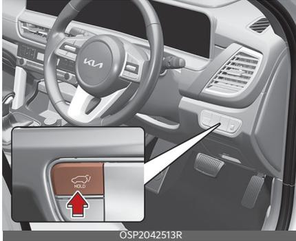
When the tailgate is closed, press the power tailgate open/close button for 1 second. The power tailgate opens with a warning sound.
