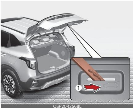
If you have to open the tailgate urgently inside the tailgate due to battery discharge, external handle failure, or other reasons.
