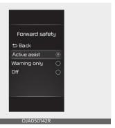
With the ignition switch or ENGINE START/STOP button in the ON position, select or deselect "User Settings → Driver Assistance → Forward safety'
