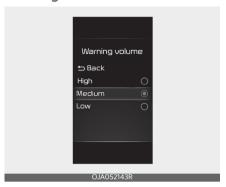
With the ignition switch or ENGINE-START/STOP button in the ON position, select 'Driver Assistance → Warning volume' from the Settings menu to change the Warning volume to 'High', 'Medium', 'Low' for Rear Cross- Traffic Safety system.
