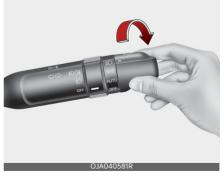
When the light switch is in the headlight position (4<sup>th</sup> position), the head, tail,
