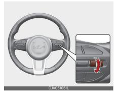
Push the SET- switch (1) down, and release it. The SET indicator light will illuminate.  Release the accelerator pedal. Vehicle speed will maintain the set speed even when the accelerator pedal is not depressed.
