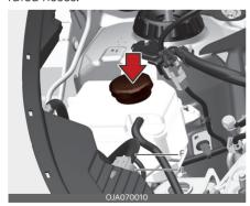
The coolant level should be filled between MAX and MIN (F and L) marks
