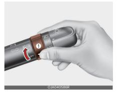
Fog lights are used to provide improved visibility when visibility is poor due to fog, rain or snow, etc. The fog lights will turn on when the fog light switch (1) is turned on after the parklight is turned on.
