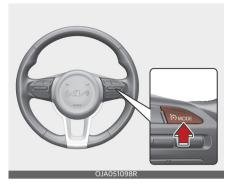
2. Push the RES+ switch up or RESswitch down, and release it at the desired speed.
