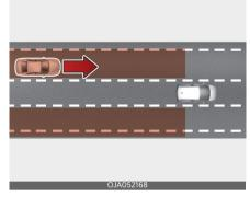
Blind-Spot Collision-Avoidance Assist help detects and informs the driver that a vehicle is approaching at high speed from the blind spot area.
