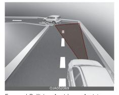
Forward Collision-Avoidance Assist may not detect other vehicles in front of you on curved roads adversely affecting the performance of the sensor. This may result in no alarm and braking when necessary.
