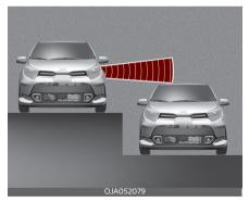
Blind-Spot Safety function may not operate properly when driving where the heights of the lanes are different. Blind-Spot Collision Warning may not detect the vehicle on a road with different lane heights (underpass joining section, grade separated intersections, etc.).
