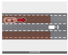
Blind-Spot Collision Warning help detects and informs the driver that a vehicle is approaching at high speed from the blind spot area.
