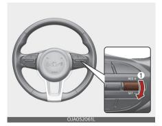
Release the accelerator pedal. Vehicle speed will maintain the set speed even when the accelerator pedal is not depressed.
