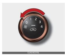
To turn off the blowers, turn the fan speed control knob to the "O" position.
