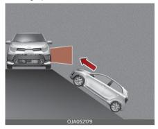
When the vehicle is on or near a slope Rear Cross-Traffic Safety may be limited when the vehicle is on a uphill or downhill slope, or near it, and may not detect the vehicle approaching from the left or right. If this occurs, the function may not warn the driver or control the brakes when necessary.
