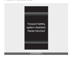
When the front windscreen where the front view camera is located, front radar cover or sensor is covered with foreign material such as snow or rain, it can reduce the detecting performance and temporarily limit or disable Forward Collision-Avoidance Assist. If this occurs the 'Forward safety system disabled. Radar blocked' warning message, and the
