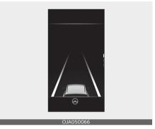
If the vehicle ahead and both lane markings are detected and your vehicle speed is below 180 km/h (110 mph), the green ( ) indicator light will illuminate on the cluster, and the function will help the vehicle stay in lane by assisting the steering wheel.
