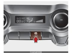
This is used to select the outside (fresh) air position or recirculated air position. To change the air intake control position, press the control button.
