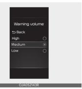
With the ignition switch or ENGINE START/STOP button in the ON position, select 'Driver Assistance → Warning volume' from the User Settings menu to change the Warning volume to 'High', 'Medium', 'Low' for Lane Keeping Assist. If you change the Warning volume, the Warning volume of other Driver Assistance systems may be changed.
