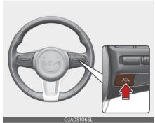
To activate/deactivate LKA, with the ignition switch or ENGINE START/STOP button in the ON position, press and hold the Lane Driving Assist button ( \( \rightarrow\)\) located on the steering wheel to turn off Lane Keeping Assist. Press and hold the button again to turn on the function.
