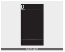
This indicator displays which Automated Manual Transmission shift lever is selected.
