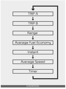
To change the trip mode, scroll the MOVE scroll switch  $(\land/\lor)$  or TRIP button in the trip computer mode.
