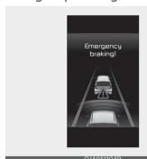
To warn the driver that emergency braking will be assisted, the 'Emergency braking' warning message will
