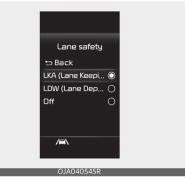
With the ignition switch or ENGINE START/STOP button in the ON position, select or deselect 'Driver Assistance → Lane safety' from the Settings menu to set whether or not to use each function.
