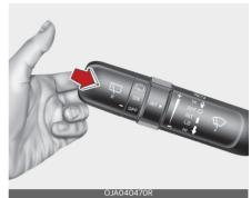
In the O (Off) position, pull the lever gently toward you to spray washer fluid on the windscreen and to run the wipers 1-3 cycles.
