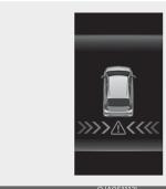
To warning the driver of an approaching vehicle from the rear left/right side of your vehicle, the outside rearview mirror will blink and a warning will appear on the cluster. At the same time, an audible warning will sound. If the Rear View Monitor system is operating, a warning will also appear on the infotainment screen.
