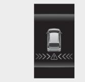
To warn the driver of an approaching vehicle from the rear left/right side of your vehicle, the warning light on the outside rearview mirror will blink and a warning will appear on the cluster. At the same time, an audible warning will sound.
