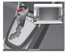
Rear View Monitor will activate when the back-up light is ON with the ignition switch ON and the shift lever in the R (Reverse) position.
