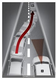
When a vehicle moves into your lane from an adjacent lane, it cannot be detected by the sensor until it is in the sensor detection range. Forward Collision-Avoidance Assist may not immediately detect the vehicle when the vehicle changes lanes abruptly. In this case, you must maintain a safe braking distance, and if necessary, steer your vehicle and depress the brake pedal to reduce your driving speed in order to maintain a safe distance.
