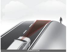
Forward Collision-Avoidance Assist may not detect other vehicles or pedestrians in front of you whilst driving uphill or downhill adversely affecting the performance of the sensors.
