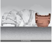
Air bags do not inflate in most rollover accidents, even though the vehicle is equipped with side air bags and curtain air bags.
