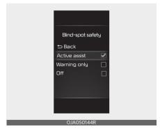
With the ignition switch or ENGINE START/STOP button in the ON position, select or deselect 'Driver Assistance → Blind-Spot Safety' from the User Settings menu to set whether or not to use each function.
