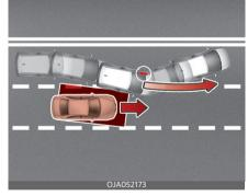
When changing lanes by detecting the lane ahead, if Blind-Spot Collision-Avoidance Assist judges that there is a collision risk with an approaching vehicle in the blind spot, Blind-Spot Collision-Avoidance Assist will help avoid collision by applying the brake.
