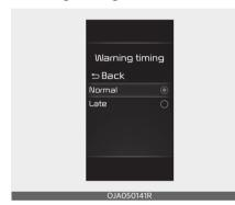
With the ignition switch or ENGINE START/STOP button in the ON position, select 'Driver Assistance → Warning timing' from the Settings menu to change the initial warning activation time for Rear Cross-Traffic Safety.
