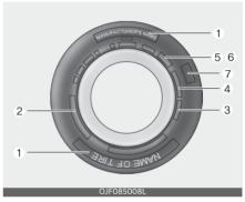
This information identifies and describes the fundamental characteristics of the tyre and also provides the tyre identification number (TIN) for safety standard certification. The TIN can be used to identify the tyre in case of a recall.
