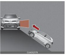
• When the vehicle is on or near a slope Rear Cross-Traffic Safety may be limited when the vehicle is on a uphill or downhill slope, or near it, and may not detect the vehicle approaching from the left or right. If this occurs, the function may not warn the driver when necessary.
