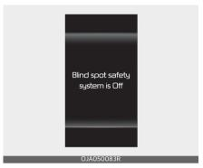
When the engine is restarted with Blind-Spot Collision Warning off, the 'Blindspot safety function is Off' message will appear on the cluster.
