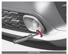
The front fog lamp can be aimed as the same manner of the head lamps aiming. With the front fog lamps and battery normal condition, aim the front fog lamps.
