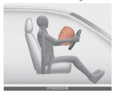
Upon deployment, tear seams molded directly into the pad covers will separate
