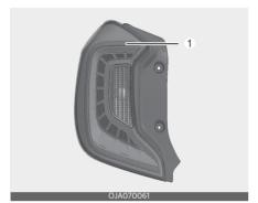
If the stop and tail lamp (LED type) (1) does not operate, have your vehicle checked by a professional workshop. Kia recommends to visit an authorised Kia dealer/service partner. The LED lamp cannot be replaced as a single component because it is an integrated unit. The LED lamp has to be replaced with the unit. A skilled technician should check or repair the stop and tail lamp (LED type), for it may damage related parts of the vehicle.
