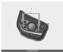
If the position lamp/daytime running lamp (LED type) (1) does not operate, have your vehicle checked by a professional workshop. Kia recommends to visit an authorised Kia dealer/service partner. The LED lamp cannot be replaced as a single component because it is an integrated unit. The LED lamp has to be replaced with the unit. A skilled technician should check or repair the position lamp/daytime running lamp (LED type), for it may damage related parts of the vehicle.
