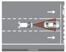
Forward Collision-Avoidance Assist is designed to help detect and monitor the vehicle ahead in the roadway and warn the driver that a collision is imminent with a warning message and an audible warning, and if necessary, apply emergency braking.
