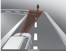
Forward Collision-Avoidance Assist may detect a vehicle or pedestrian in the next lane or outside the lane when driving on a curved road. If this occurs, the unnecessarily alarm the driver and apply the brake.
