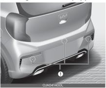
Reverse Parking Distance Warning assists the driver during backward movement of the vehicle by chiming if any object is sensed within a distance of 100 cm (40 in.) behind the vehicle.
