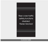
When the rear bumper around the rearside radar or sensor is covered with foreign matters, such as snow or rain, or installing a trailer or carrier, it can reduce the detecting performance and temporarily limit or disable Rear Cross-Traffic Safety.
