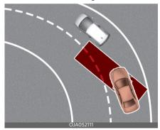
Blind-Spot Safety function may not operate properly when driving on the curved road. Blind-Spot Collision-Avoidance Assist may recognize the vehicle in the same lane.
