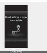
When the outside rearview mirror warning light is not working properly, the 'Check side view mirror warning light'
