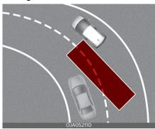
Blind-Spot Safety function may not operate properly when driving on a curved road. Blind-Spot Collision-Avoidance Assist may not detect the vehicle in the next lane.
