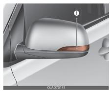
If the side repeater lamp (LED type) (1) does not operate, have your vehicle checked by a professional workshop. Kia recommends to visit an authorised Kia dealer/service partner. The LED lamp cannot be replaced as a single component because it is an integrated unit. The LED lamp has to be replaced with the unit. A skilled technician should check or repair the side repeater lamp (LED type), for it may damage related parts of the vehicle.
