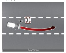
Lane Keeping Assist is designed to help detect the lane markers (or road edges) whilst driving over a certain speed. Lane Keeping Assist will warn the driver if the vehicle leaves the lane without using the turn signal, or will automatically assist the driver's steering to help prevent the vehicle from departing the lane.
