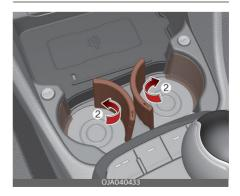
To use the cup holder space as a storage compartment, turn the half part of the cup holder (2) to the direction of the arrow.
