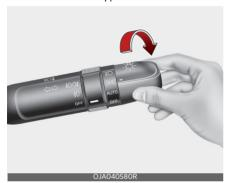
When the light switch is in the parking light position (3<sup>rd</sup> position), the tail position, license and instrument panel lights will turn ON.
