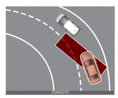
Blind-Spot Safety function may not operate properly when driving on the curved road. Blind-Spot Collision Warning may recognize the vehicle in the same lane.
