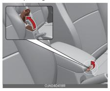
To open the centre console storage pull up the lever.
