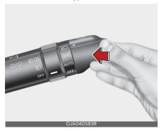
To turn on the high beam headlights, push the lever away from you when the
