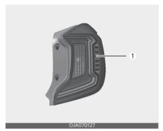
If the stop lamp (LED type) (1) does not operate, have your vehicle checked by a professional workshop. Kia recommends to visit an authorised Kia dealer/service partner. The LED lamp cannot be replaced as a single component because it is an integrated unit. The LED lamp has to be replaced with the unit. A skilled technician should check or repair the stop lamp (LED type), for it may damage related parts of the vehicle.
