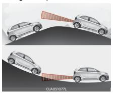
Blind-Spot Safety function may not operate properly when driving on a slope. Blind-Spot Collision Warning may not detect the vehicle in the next lane or may incorrectly detect the ground or structure.
