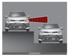
Blind-Spot Safety function may not operate properly when driving where the heights of the lanes are different. Blind-Spot Collision-Avoidance Assist may not detect the vehicle on a road with different lane heights (underpass joining section, grade separated intersections, etc.). Always pay attention to road and driving conditions whilst driving.
