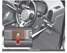
The Electronic Stability Control (ESC) system is designed to stabilize the vehicle during cornering manoeuvres. ESC
