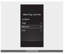
With the ignition switch or ENGINE-START/STOP button in the ON position, select 'Driver Assistance → Warning volume' from the Settingsmenu to change the Warning volume to 'High', 'Medium', 'Low' for Rear Cross- Traffic Safety system. If you change the Warning volume, the Warning volume of other Driver Assistance systems may change.
