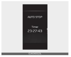
This mode displays the elapsed time of Auto stop by "Idle stop and go system". For more details, refer to "ISG (Idle Stop and Go) system (if equipped)" on page 6-17.
