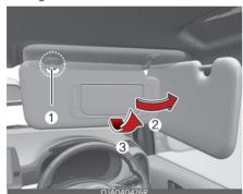
To use the sunvisor, pull it downward. To use the sunvisor for the side window, pull it downward, unsnap it from the bracket (1) and swing it to the side (2). To use the vanity mirror, pull down the visor and slide the mirror cover (3). The ticket holder (4) is provided for holding a tollgate ticket. (if equipped)
