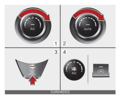
If the mosition is selected, lowerfan speed is adjusted to a higher fanspeed.
