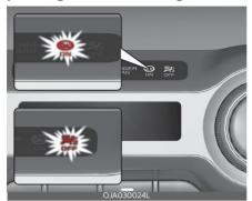
To deactivate the passenger's front air bag, insert the master key into the passenger's front air bag ON/OFF switch and turn it to the OFF position. The passenger's front air bag OFF indicator (()) will illuminate and stay on until the passenger's front air bag is reactivated. To reactivate the passenger's front air bag, insert the master key into the passenger's front air bag ON/OFF switch and turn it to the ON position.
