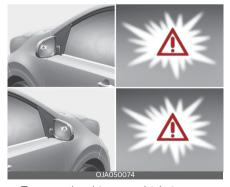
To warn the driver a vehicle is detected, the warning light on the outside rearview mirror and head-up display (if equipped) will illuminate
