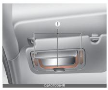
If the vanity mirror lamp (LED type) (1) does not operate, have your vehicle checked by a professional workshop. Kia recommends to visit an authorised Kia dealer/service partner. The LED lamp cannot be replaced as a single component because it is an integrated unit. The LED lamp has to be replaced with the unit. A skilled technician should check or repair the vanity mirror lamp (LED type), for it may damage related parts of the vehicle.
