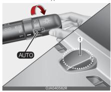
When the light switch is in the AUTO light position, the taillights and head-lights will be turned ON or OFF automatically depending on the amount of light outside the vehicle.
