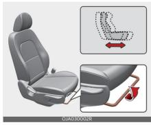
Adjust the seat before driving, and make sure the seat is locked securely by trying to move forward and rearward without using the lever. If the seat moves, it is not locked properly.
