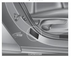
The Certification/Tyre label is found on the front edge of the RH (or LH) "B" pillar. The label shows the size of your original tyres and inflation pressures needed to obtain the gross weight capacity of your vehicle.
