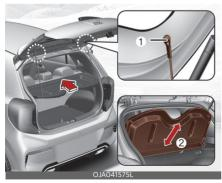
2. whilst lifting the cover up, hold the area near the front slots. Then, pull up
