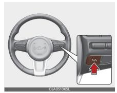
With the ignition switch or the ENGINE START/STOP button in the ON position, press the Lane Driving Assist button located on the steering wheel to turn on Lane Following Assist. The white or green ( ) indicator light will illuminate on the cluster.
