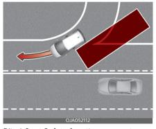
Blind-Spot Safety function may not operate properly when driving where the road merges or divides. Blind-Spot Collision Warning may not detect the vehicle in the next lane.
