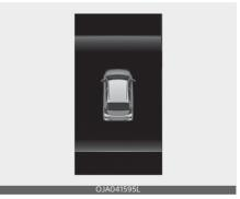
The warning message (for Type B, C cluster) will appear on the LCD display when bonnet is open.
