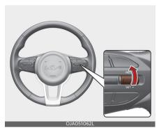
To resume Manual Speed Limit Assist after Manual Speed Limit Assist was paused, operate the RES+, RES- switch. If you press the RES+ switch up or RES-switch down, vehicle speed will be set to the current speed on the cluster.
