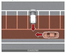
• When the vehicle is parked rearward Rear Cross-Traffic Safety may detect vehicles passing by behind you when parking backwards into a parking space. If this occurs, the function may unnecessarily warn the driver and control the brake.
