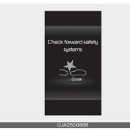
When Forward Collision-Avoidance Assist is not working properly, the 'Check forward safety system' warning message will appear, and the
