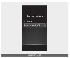
With the ignition switch or ENGINE START/STOP button in the ON position, select 'Driver Assistance → Parking safety → Rear cross-traffic safety' from
