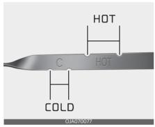
4. If the fluid level is checked in cold condition [fluid temperature 20~30°C (68~86°F)], add the fluid to the "COLD" line and then recheck the fluid level according to the above step 2.
