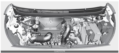
\* The actual engine room in the vehicle may differ from the illustration. 1. Engine coolant reservoir 8-40, 8-42 2. Engine oil filler cap 8-37 3. Brake/clutch fluid reservoir 8-45 4. Air cleaner 8-49, 8-50 5. Fuse box 8-71 6. Negative battery terminal 8-56 8-56 7. Positive battery terminal 8. Engine oil dipstick 8-37 8-40, 8-42 9. Radiator cap
