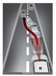
When a vehicle in front of you merges out of the lane, Forward Collision-Avoidance Assist may not immediately detect the vehicle that is now in front of you. In this case, you must maintain a safe braking distance, and if necessary, steer your vehicle and depress the brake pedal to reduce your driving speed in order to maintain a safe distance.
