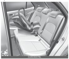
A rearward-facing Child Restraint System provides restraint with the seating surface against the back of the child. The harness system holds the child in place, and in an accident, acts to keep the child positioned in the Child Restraint Systems and reduce the stress to the fragile neck and spinal cord.
