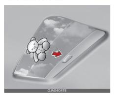
If the sunroof glass senses any obstacle whilst it is closing automatically, it will reverse direction then stop at a certain position.
