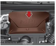
1. Loosen the air cleaner cover attaching clips.
