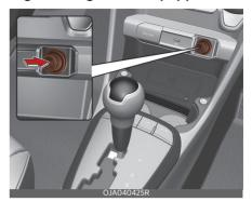
For the cigarette lighter to work, the ignition switch must be in the ACC position or the ON position.
