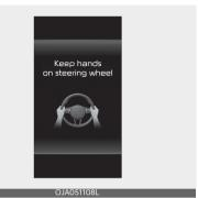
If the driver takes their hands off the steering wheel for several seconds, the 'Keep hands on steering wheel' warning message will appear on the cluster, and an audible warning will sound in stages.
