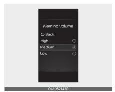
With the ignition switch or ENGINE START/STOP button in the ON position, select 'Driver Assistance → Warning volume' from the Settings menu to change
