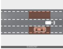
Blind-Spot Collision Warning help detects and informs the driver that a vehicle is in the blind spot.
