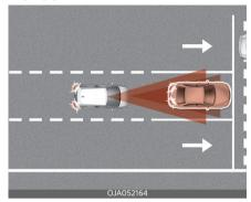
Forward Collision-Avoidance Assist is designed to help detect and monitor the vehicle ahead or help detect a pedestrian in the roadway and warn the driver that a collision is imminent with a warning message and an audible warning, and if necessary, apply emergency braking.
