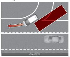
Blind-Spot Safety function may not operate properly when driving where the road merges or divides. Blind-Spot Collision-Avoidance Assist may not detect the vehicle in the next lane. Always pay attention to road and driving conditions whilst driving.
