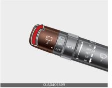
Turn the wiper lever switch upwards twice to spray rear washer fluid and to run the rear wipers 1~3 cycles.
