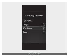
With the ignition switch or ENGINE START/STOP button in the ON position, select 'Driver Assistance → Warning volume' from the User Settings menu to
