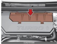
1. Pull the air filter cap to open.
