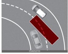
Blind-Spot Safety function may not operate properly when driving on a curved road. Blind-Spot Collision Warning may not detect the vehicle in the next lane.
