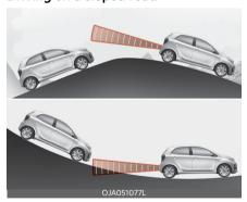
Blind-Spot Safety function may not operate properly when driving on a slope. Blind-Spot Collision-Avoidance Assist may not detect the vehicle in the next lane or may incorrectly detect the ground or structure.
