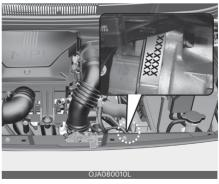
The engine number is stamped on the engine block as shown in the drawing.
