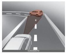
Forward Collision-Avoidance Assist may detect a vehicle in the next lane or outside the lane when driving on a curved road. If this occurs, the unnecessarily alarm the driver and apply the brake. Always check the traffic conditions around the vehicle.
