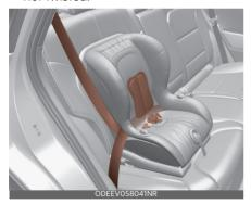
Fasten the lap/shoulder belt latch into the buckle. Listen for the distinct "click" sound. Position the release button so that it is easy to access in case of an emergency.
