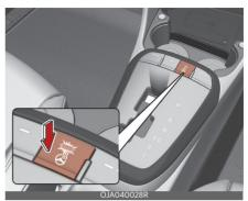
When the ignition switch is in the ON position, pressing the heated steering wheel button warms the steering wheel. The indicator on the button will illuminate.
