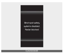
When the rear bumper around the rear corner radar or sensor is covered with foreign material, such as snow or rain, or installing a trailer or carrier, it can reduce the detecting performance and temporarily limit or disable Blind-Spot Safety function.
