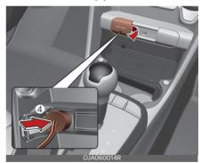
9. With the ENGINE START/STOP button position on or ignition switch position on, switch on the compressor and let it run for approximately 5~7 minutes to fill the sealant up to roper pressure. The inflation pressure of the tyre after filling is unimportant and will be checked/corrected later.
