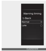
With the ignition switch or ENGINE START/STOP button in the ON position, select 'Driver Assistance → Warning timing' from the Settings menu to change the initial warning activation time for Rear Cross-Traffic Safety.
