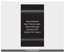
Check the pressure of all tyre and inflate to the proper pressure according to procedures, and if required, replace or repair the tyre.
