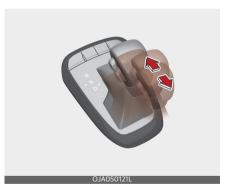
Whether the vehicle is stationary or in motion, Manual shift mode is selected by pushing the shift lever from the D (Drive) position into the manual gate (M). To return to D (Drive) range operation, push the shift lever back into the main gate.In Manual shift mode, moving the shift lever backwards and forwards will allow you to select the desired range of gears for the current driving conditions.
