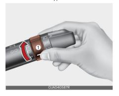
To turn the rear fog lights on, turn the rear fog light switch (1) to the on position when the headlight is turned on.
