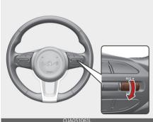
If any method other than the \( \)\ \( \)\ MODE button was used to cancel cruising speed and the system is still activated, the most recent set speed will automatically resume when you move the lever up (to RES+).
