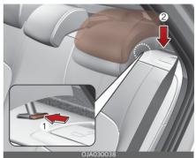
To remove the headrest, raise it as far as it can go then press the release button (1) whilst pulling upward (2).
