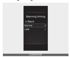
With the ignition switch or ENGINE START/STOP button in the ON position, select 'Driver Assistance → Warning timing' from the Settings menu to change the initial warning activation time for Blind-Spot Safety function.
