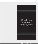
When Rear Cross-Traffic Safety is not working properly, the 'Check Rear Cross-Traffic Safety system' warning message will appear on the cluster, and Rear Cross-Traffic Collision-Avoidance Assist will turn off automatically or it will be limited. In this case, have the vehicle inspected by a professional workshop. Kia recommends to visit an authorised Kia dealer/service partner.
