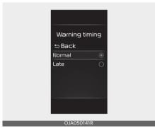
With the ignition switch or ENGINE START/STOP button in the ON position, select 'Driver Assistance → Warning timing' from the User Settings menu to change the initial warning activation time for Forward Collision-Avoidance Assist.
