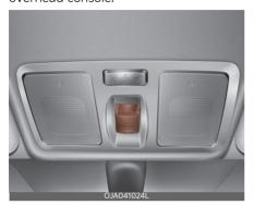
The sunroof can only be operated when the ignition switch or Engine Start/Stop button is in the ON position. The sunroof can be operated for approximately 30 seconds after the ignition switch or Engine Start/Stop button is in the ACC or LOCK/OFF position.
