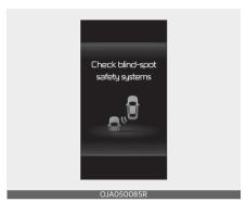
When Blind-Spot Safety function is not working properly, the 'Check Blind-spot safety system' warning message will appear on the cluster, and Blind-Spot Collision Warning will turn off automatically, or it will be limited. In this case, have your vehicle inspected by a professional workshop. Kia recommends to contact an authorised Kia dealer/service partner.
