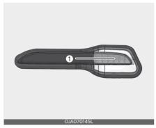
If the rear fog lamp (LED type) (1) does not operate, have your vehicle checked by a professional workshop. Kia recommends to visit an authorised Kia dealer/ service partner. The LED lamp cannot be replaced as a single component because it is an integrated unit. The LED lamp has to be replaced with the unit. A skilled technician should check or repair the rear fog lamp (LED type), for it may damage related parts of the vehicle.
