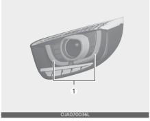
If the daytime running lamp (LED type) (1) does not operate, have your vehicle checked by a professional workshop. Kia recommends to visit an authorised Kia dealer/service partner. The LED lamp cannot be replaced as a single component because it is an integrated unit. The LED lamp has to be replaced with the unit. A skilled technician should check or repair the daytime running lamp (LED type), for it may damage related parts of the vehicle.
