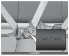
When using the rear centre seat belt, the buckle with the "CENTRE" mark must be used.
