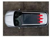
Securing a child restraint system with "ISOFIX anchorage system" and "Toptether anchorage" system [3]. System [3].
