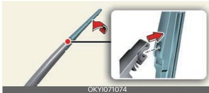
3. Install the new blade assembly by inserting the centre part into the slot in the wiper arm until it clicks into place.
