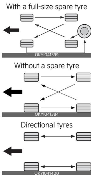
To equalize tread wear, it is recommended that the tyres be rotated every 10,000 km (6,500 miles) or sooner if irregular wear develops.
