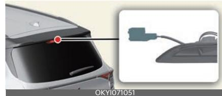
3. Remove the spoiler bolts fixing the high mounted stop lamp using a T-wrench and pull out the spoiler.
