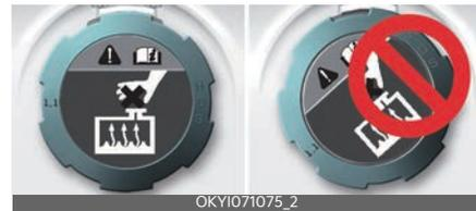
2. Make sure that the tiny protrusions inside the coolant cap are securely interlocked.
