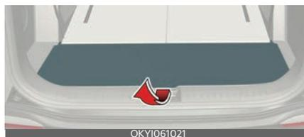
2. Find the spare tyre fixing bolt cover and remove the cover. If necessary, separate the tool case only after removing the clamp.
