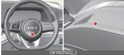
The indications of the system's presence are the letters "AIR BAG" intagliated on the air bag pad cover in the steering wheel and the passenger's side front panel pad above the glove box.
