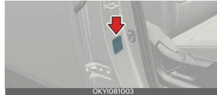
The vehicle certification label attached on the centre pillar as shown gives the vehicle identification number (VIN).
