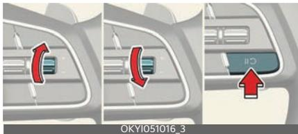
To resume Manual Speed Limit Assist after the function was paused, operate the +, - switch up or - switch down, vehicle speed will be set to the current speed on the cluster.
