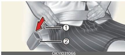
2. Check to make sure the belt is properly locked and that the belt is not twisted. With a 2-point static type seat belt, the length must be adjusted
