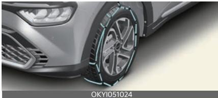
Since the sidewalls of radial tyres are thinner, they can be damaged by mounting some types of snow chains on them. Therefore, the use of snow tyres is recommended instead of snow chains. Do not mount tyre chains on vehicles equipped with aluminium wheels; snow chains may cause damage to the wheels. If snow chains must be used, use fabric-type chains or wire-type chains with a thickness of less than 15 mm (0.59 inches).
