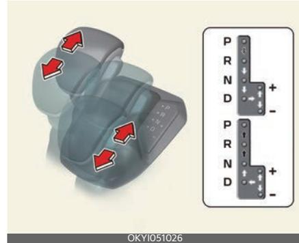
▬➔ Depress the brake pedal and the lock release button when shifting.
