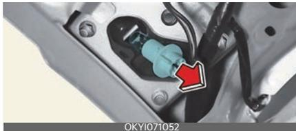
5. Insert a new bulb by inserting it into the socket and rotating it until it locks into place.
