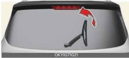
2. Lift up the wiper blade, and pull the blade to remove it.
