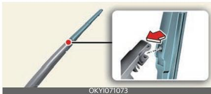
4. Make sure the blade assembly is installed firmly by trying to pull it slightly.
