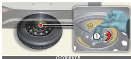
5. After the spare tyre reaches the ground, continue to turn the wrench counterclockwise, and draw the spare tyre outside. Never rotate the wrench excessively, otherwise the spare tyre carrier may be damaged.
