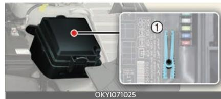
4. Check the removed fuse; replace it if it is blown. Spare fuses are provided in the instrument panel fuse panel (or in the engine compartment fuse panel).
