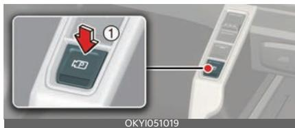
Press the Parking/View button (1) to turn on or off Rear View Monitor.
