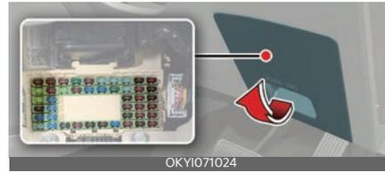
3. Pull the suspected fuse straight out. Use the removal tool provided in the main fuse box in the engine compartment.
