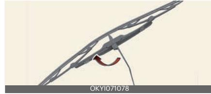
2. Compress the clip and slide the blade assembly downward.
