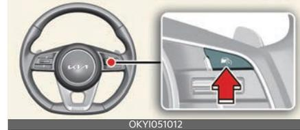
Press the Driving Assist (⚠) button to turn Manual Speed Limit Assist off. The Speed Limit indicator (S LIMIT) will go off.
