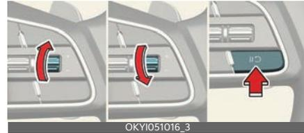
Operate the +, - switch or (||◁) button. If you push the + switch up or - switch down, vehicle speed will be set to the current speed on the cluster. If you press the (||◁) button, vehicle speed will resume to the preset speed. Vehicle speed must be above 30 km/h (20 mph) for Cruise Control to resume.
