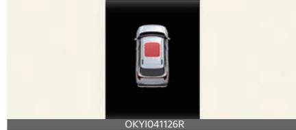
If the driver turns off the engine when the sunroof is not fully closed, the warning chime will sound for several seconds and the sunroof open warning will appear on the cluster LCD display.
