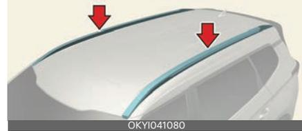
Do not load cargo on roof. The roof rack is not intended for load carriage and it is for aesthetics only.
