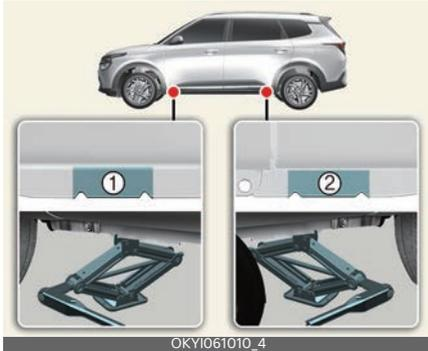
9. Insert the jack handle into the jack and turn it clockwise. Raise the vehicle until the tyre just clears the ground. Make sure the vehicle is stable before removing the wheel lug nuts.
