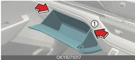
2. Remove the climate control air filter cover by pulling out both sides of the cover.
