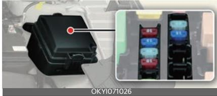
When the blade type fuse is disconnected, remove it by using the clip designed for changing fuses located in the engine room fuse box. Upon removal, securely insert reserve fuse of equal quantity.
