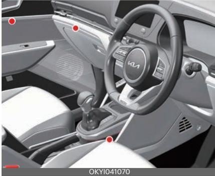
The ambient lights are applied to the front crash pad, doors, and the centre console.
