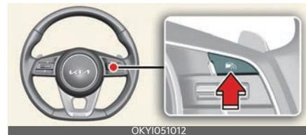
Press the Driving Assist (Ⓢ) button to turn Cruise Control off. The Cruise (Ⓢ) indicator will go off. Always press the Driving Assist button to turn Cruise Control off when not in use.
