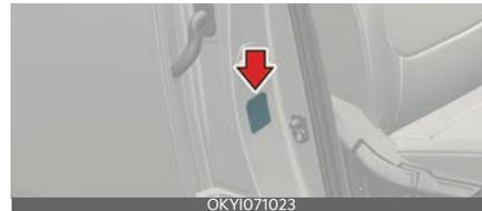
The tyre label located on the centre pillar as shown gives the tyre pressures recommended for your vehicle. The tyres supplied on your new vehicle are chosen to provide the best performance for normal driving.
