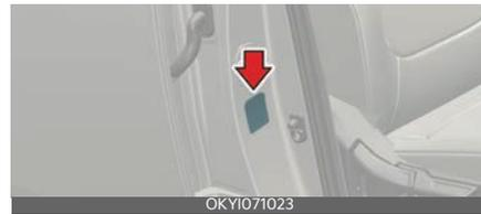
All specifications (sizes and pressures) can be found on a label attached to the driver's side centre pillar.
