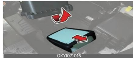
4. Lock the cover with the cover attaching clips. Assemble in reverse order. Replace the filter according to the Maintenance Schedule.
