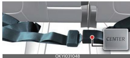
6. When you want to release the seat belt, press the button (1) in the locking buckle.
