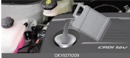
Use a funnel to help prevent oil from being spilled on engine components. Use only the specified engine oil. (Refer to "Recommended lubricants and capacities" on page 8-6.)
