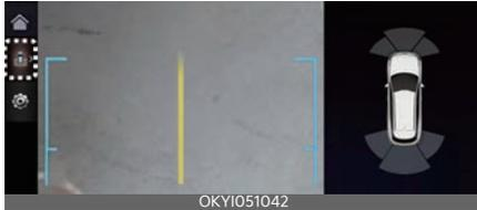
Rear top view shows the distance from the vehicle or the object in the back of your vehicle whilst parking.
