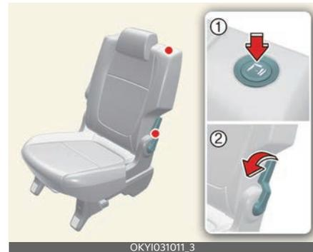
5. Back of the seatback will slightly go up, then lift up the 2nd row seat and set to upright position (vertical position).
