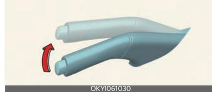
Check the stroke of the parking brake by counting the number of "clicks" heard whilst fully applying it from the released position. Also, the parking brake alone should securely hold the vehicle on a fairly steep grade. If the stroke is more or less than specified, we recommend that the system be inspected by an authorised kia dealer.
