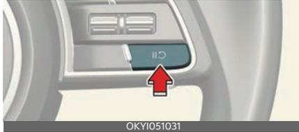
Press the (||) button to temporarily pause the set speed limit. The set speed limit will turn off but the Speed Limit indicator (S LIMIT) will stay on.
