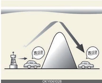
AM broadcasts can be received at greater distances than FM broadcasts. This is because AM radio waves are transmitted at low frequencies. These long distance, low frequency radio waves can follow the curvature of the earth rather than travelling straight. In addition, they curve around obstructions resulting in better signal coverage.
