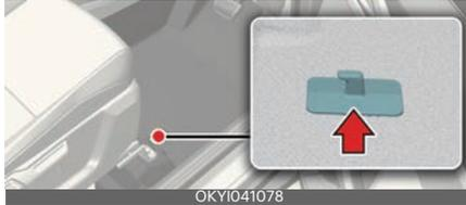
Make sure the floor mat attaches to the anchors to keep the floor mat from sliding forward.
