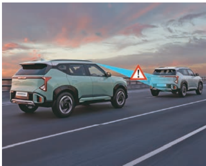
Front Collision Warning and Avoidance Assist (FCW& FCA)
