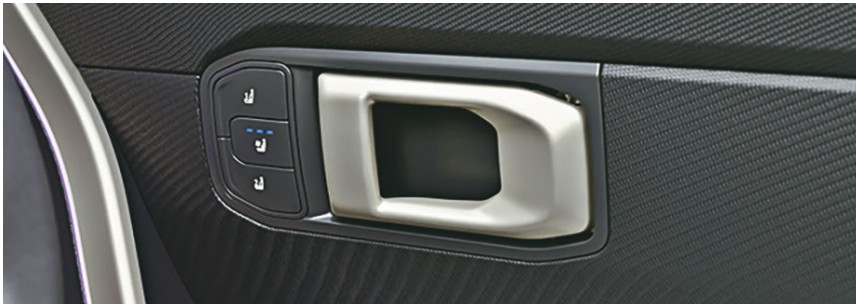
Adaptive Integrated Memory System (Driver Seat & ORVMs)
