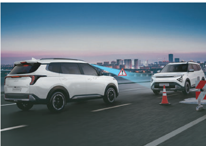
Forward Collision Avoidance Assist - Direct Oncoming (FCA-DO)
