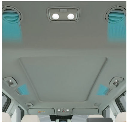
Roof Mounted Air Vents
