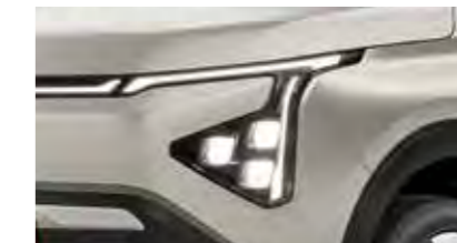
Star Map LED Connected DRLs with Integrated Turn Signals
