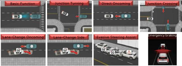
FCA can detect a vehicle, a motorcyclist, pedestrian, or cyclist ahead on the road, may warn you of a possible collision with a warning message, a warning sound and may assist with braking.
