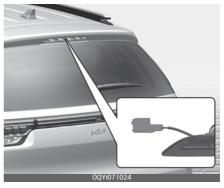
4. Remove the bulb holder bracket from the assembly.
