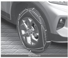
Since the sidewalls of radial tyres are thinner, they can be damaged by mounting some tupes of snow chains on them. Therefore, the use of snow tyres is recommended instead of snow chains. Do not mount ture chains on vehicles equipped with aluminium wheels; snow chains may cause damage to the wheels. If snow chains must be used, use wire-type chains with a thickness of less than 15 mm. Damage to your vehicle caused by improper snow chain use is not covered by your vehicle manufacturers warranty.
