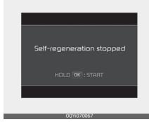
The self regeneration process stops if any of the self regeneration conditions is cancelled. If the self regeneration process is cancelled automatically, the system maintains "Self regeneration stopped" message.
