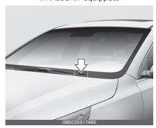
The VIN is also on a plate attached to the top of the dashboard. The number on the plate can easily be seen through the windscreen from outside.
