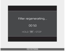
If the self regeneration mode starts, the message "Filter regenerating..." and the remaining time appears. It takes around 30~60 minutes.
