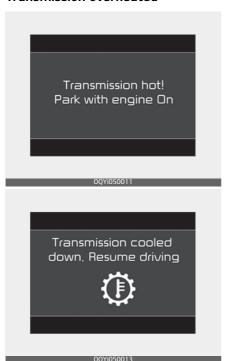
When driving on muddy and sandy roads under the severe condition, the transmission could be overheated.
