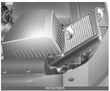
4. Lock the cover with the cover attaching clips.
