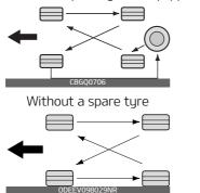
Rotate radial tyres that have an asymmetric tread pattern only from front to rear and not from right to left.
