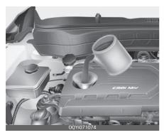
Use only the specified engine oil. (Refer to "Recommended lubricants and capacities" on page 9-6.)
