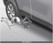
9. Loosen the wheel nuts and remove them with your fingers. Slide the wheel off the studs and lay it flat so it cannot roll away. To put the wheel on the hub, pick up the spare tyre, line up the holes with the studs and slide the wheel onto them.
