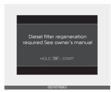
If the system still needs the self regeneration process after cancelling the operation, the warning message appears. (Diesel filter regeneration required.)
