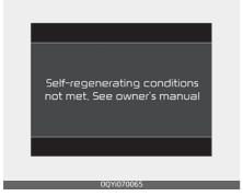
Under below condition, Diesel Catalyst regeneration process may be interrupted. (Engine RPM drops to idle state)
