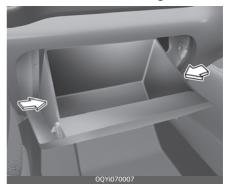
3. Remove the climate control air filter cover by pulling out left side of the cover.
