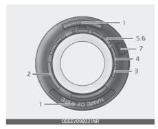
The TIN can be used to identify the tyre in case of a recall.
