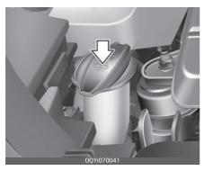
The reservoir is translucent so that you can check the level with a quick visual inspection.
