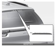
2. Remove the three round head cap nut fixing the high mounted stop lamp using a wrench. 3. Pull out the high mounted stop lamp assembly and unplug the connector.
