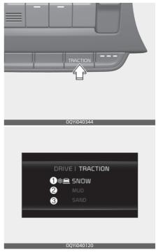
If you press the "TRACTION" mode button, the Traction control mode can be selected. You can toggle
