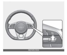
Accelerate to the desired speed, which must be more than 30 km/h.
