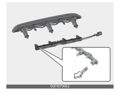
6. Insert a new bulb in the socket.
