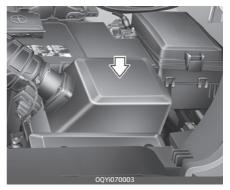
You can clean the filter when inspecting the air cleaner compartment. Clean the filter by using compressed air.
