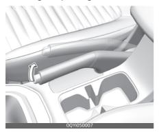
Check the stroke of the parking brake by counting the number of "clicks" heard whilst fully applying it from the released position. Also, the parking brake alone should securely hold the vehicle on a fairly steep grade. If the stroke is more or less than specified, we recommend that the system be inspected by an authorised kia dealer.
