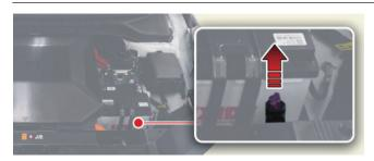
If the charging cable does not detach due to battery discharge and failure of the electric wires, open the hood and slightly pull the emergency cable as shown above. The charging connector will then unlock.
