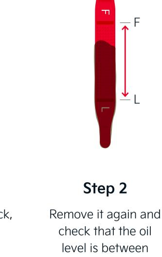
Open the bonnet and find the dipstick underneath the engine. Petrol
