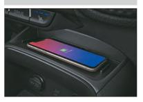
For charging a compatible smartphone wirelessly on the pad
