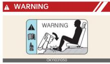
Prevent injury of 3rd row passenger foot during 2nd row unfolding and during Ingress/Engress for 3rd row seat.
