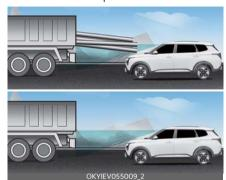
In the following cases, the vehicle in front cannot be detected by the sensor. Always pay attention to the road and driving conditions and drive safely. If necessary, adjust your vehicle speed.
