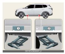
10.Insert the jack handle into the jack and turn it clockwise. Raise the vehicle until the tyre just clears the ground. Make sure the vehicle is stable before removing the wheel lug nuts.
