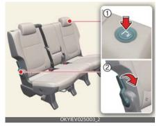
Back of the seatback will slightly go up, then lift up the 2nd row seat and set to upright position (vertical position).
