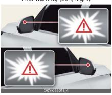
The warning light on the cluster, the outside rear view mirror and head-up display (if equipped) will appear when the vehicle on both lanes is detected from the rear.
