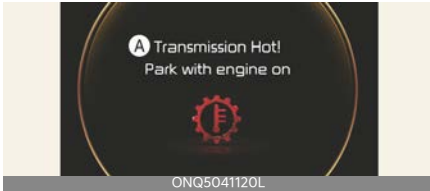
A: Transmission Hot! Park with engine on
