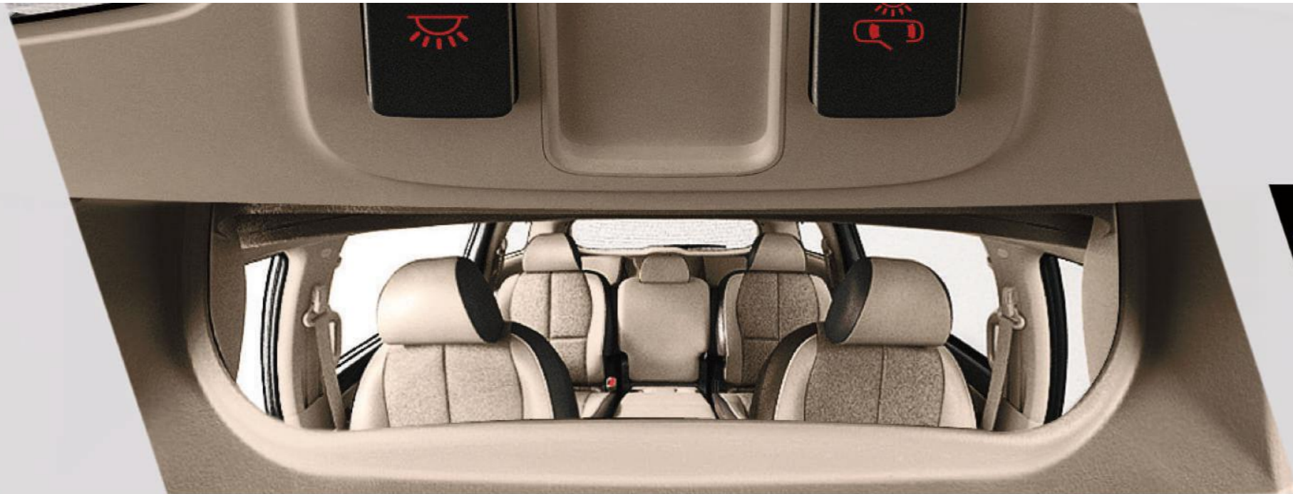
Conversation Mirror Looking over your shoulder while driving can be dangerous. Talk to rear-seat passengers without turning your head.
