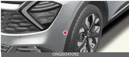
Rear side ultrasonic sensors
