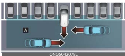
[A]: Rear Cross-Traffic Collision Warning operating range
