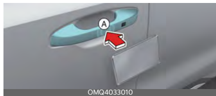
A: Door handle authentication pad B: Card key NFC antenna
