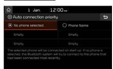
When the engine is running, the selected Bluetooth device is automatically connected. If you fail to connect the selected device, the previously-connected device is automatically connected, and if it also fails, then it tries to connect all paired devices sequentially.
