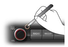
The System Reset function restores the system when it is not operating correctly. Press and hold the RESET key for a second or longer (it is recommended that you press the RESET key using a tool, such as a pin or a paperclip).
