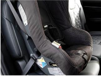
Installing a child restraint system with a lap/shoulder belt [3].
