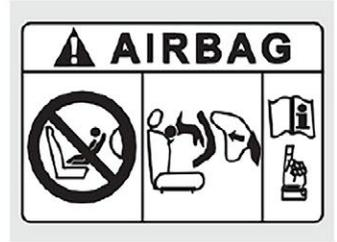
Never place a rear facing child restraint in the front passenger seat, unless the passenger-side air bag is deactivated. An inflated passenger-side air bag could impact the rear-facing child restraint and kill the child.
