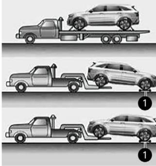
When being towed by a commercial tow truck and wheel dollies are not used, the front of the vehicle should always be lifted, not the rear.
