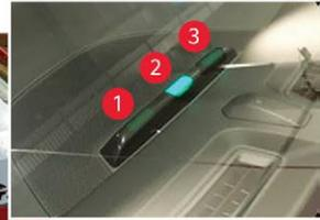
When charging the high voltage battery, the charge level can be checked from outside the vehicle.
