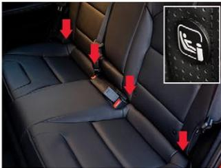
ISOFIX anchorages are located between the seatback and the seat cushion of the rear seat left and right outboard seating positions, indicated by the symbols.
