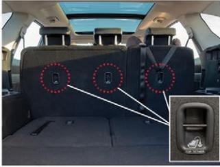
Securing a child restraint system seat with "Top-tether Anchorage" system.
