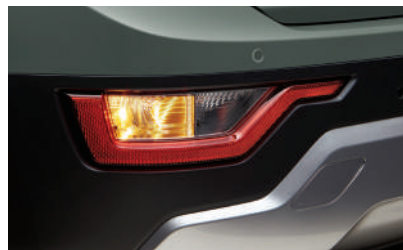
Bulb turn signal lamps (EX)
