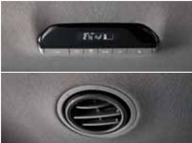
Rear Ventilation System
